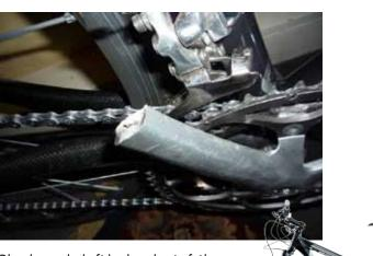
Bicycle crank shaft broken due to fatigue
